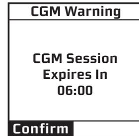
During this time your pump will continue to receive CGM readings. Once the final 30 minutes ends, you will be prompted that your CGM session has ended. Press **OK** to confirm the CGM Warning and return to the CGM Menu screen. You will no longer receive CGM readings on your pump until you replace the Sensor and begin a new CGM session (see *Chapter 4* in *Section II*).
