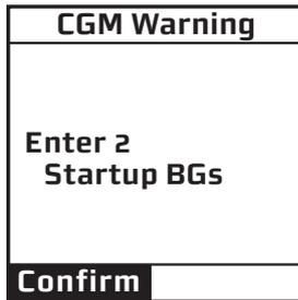
When the 2-hour CGM startup period ends, you will be prompted to enter 2 separate fingerstick BG values in your pump. Press **OK** to confirm the Warning.
