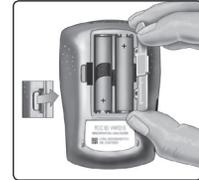
Lift both batteries out of the compartment by pulling up on the ribbon.
