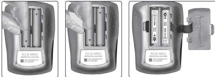
Locate the plus (+) signs inside the battery compartment and on your fresh AAA alkaline batteries. Take the plus (+) end of one battery and insert it underneath the plastic tab that sticks out at the top of the compartment. Then push down on the minus (-) end of the battery until it clicks into place.
