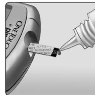
Touch and hold the hanging drop of control solution to the narrow channel in the top edge of the test strip. Make sure the confirmation window fills completely. Control Solution should not be applied to the flat face of the test strip.
