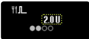
**4/7:** Each bolus amount set is displayed to you on the screen. When you have entered the bolus amount required, you have to wait 4 seconds. The elapsed time is displayed to you by dots turning gray.
