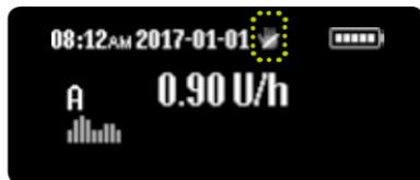
**4/5:** The status screen appears. The activated access lock function is visualized by an access lock icon at the top of the screen.
