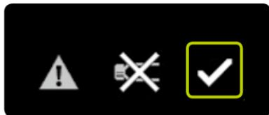
The “No insulin” alarm appears if after a threaded rod return no priming procedure is performed within 5 minutes or if the priming procedure failed. The “No insulin” alarm only appears if the insulin pump is in run mode. Confirm by tapping
