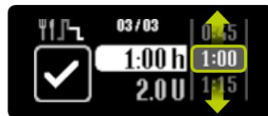
**6/8:** Select the extension time during which you wish to deliver the remaining portion of the bolus amount (extended portion). Extension time can be set from 15 minutes to 12 hours in steps of 15 minutes.
