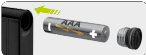
**1/11:** Insert a new AAA alkaline battery (LR03). Make sure the negative pole of the battery is inserted first. On the back of the insulin pump you will see a picture showing how to insert the battery.
