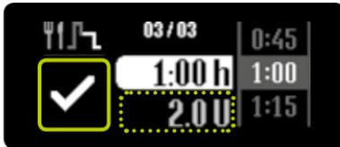
**7/8:** The bolus amount of the extended portion is displayed in gray below the extension time selected. The YpsoPump® starts bolus delivery after confirmation by tapping . The insulin pump vibrates briefly.
