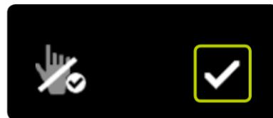
**3/5:** Confirm by tapping
