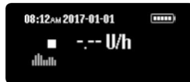
**8/8:** The status screen appears. The Ypsopump® is in stop mode. To start insulin delivery switch the insulin pump into run mode. The difference between run mode and stop mode is explained on page 25.
