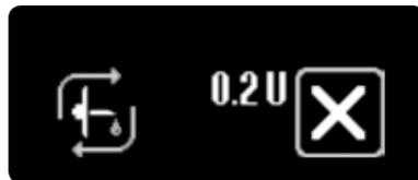
**4/4:** During the priming procedure, the screen counts the delivered priming volume upwards until the set value has been reached. You can cancel the priming procedure at any time by tapping
