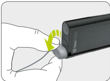
**6/7:** Disconnect the infusion set by turning the adapter on the YpsoPump® counterclockwise until it stops.
