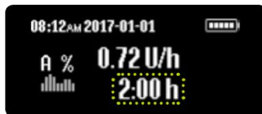
**7/7:** In addition, the period of time remaining and the selected percentage of the basal rate are displayed alternately under the basal rate value.
