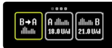
**3/4:** If basal rate profile B is active, tap the “Switch to basal rate profile A” icon.
