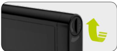
**5/5:** Lock the battery compartment by inserting a coin in the groove of the battery compartment lid and turning it clockwise until it stops. When the battery has been inserted, the mylife™ icon appears first, followed by the status screen or welcome screen. The latter appears if the battery has been removed during a threaded rod return or during a self-test after starting up from the storage status. Change the battery compartment lid every three months to minimize signs of wear.
