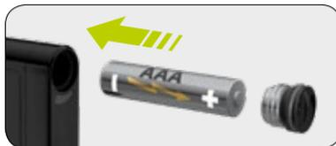
**4/5:** Insert a new, size AAA, alkaline battery (LR03). Make sure the negative pole of the battery is inserted first. On the back of the insulin pump you will see a picture showing how to insert the battery. You can obtain replacement batteries from the usual battery sales outlets.
