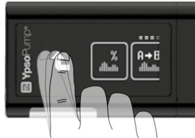
Using your finger, swipe up or down through the values displayed. In this way you can increase or reduce a value. You can also tap the upper or lower value directly in order to increase or reduce it by one unit. The value selected is always displayed at the center of the visible values and it has a gray background. Do not use the device if it shows visible signs of damage. If the device no longer responds to touch, stop using it. In such a case, contact Customer Service without delay.
