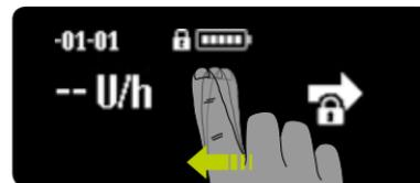
**3/6:** Swipe to the left to unlock the status screen and the main menu. Three icons appear numbered 1, 2 and 3 (unlock screen).
