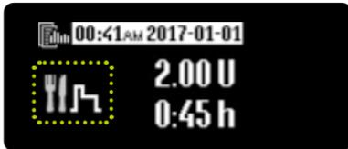
**4/4:** Example of a combination bolus: the display of the percentage value of the immediate portion alternates with the display of the extension time of the extended portion at intervals of 2 seconds.
