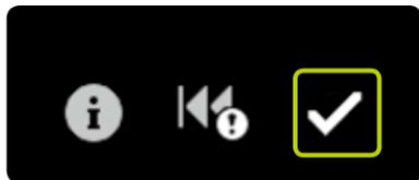
The “Threaded rod return not completed” warning appears if it has not yet been possible to perform the threaded rod return function properly. The warning can occur on account of dirt (sand, dried insulin, etc.) in the cartridge compartment or generally if the drive has a mechanical fault. This fault can also be triggered by touching the threaded rod with an object when the threaded rod is returning.
