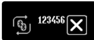
**4/6:** A six-digit number code appears on the screen of the YpsoPump® and the arrows rotate. Enter this code on your Bluetooth® enabled device.
