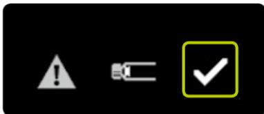
The “Cartridge empty” alarm appears if the cartridge contains 0.0 U insulin. Confirm by tapping . Change the cartridge in accordance with the procedure on page 95.
