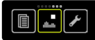
**1/3:** Open the main menu, swipe to the left and tap the “Stop mode/switch to run mode” icon.
