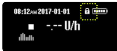
**2/6:** The YpsoPump® has a screen lock. It is visualized by a padlock icon at the top right of the screen, next to the battery charge indicator.
