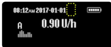
**4/5:** The status screen appears. The access lock icon at the top of the screen disappears. All icons are now active and the functions can be operated again.
