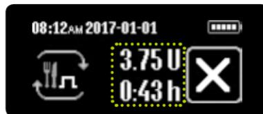
**6/6:** The YpsoPump® counts down the remaining units on the status screen. In addition, the remaining extension time of the extended bolus is displayed. You can cancel a bolus in progress at any time by tapping . Cancellation must always be confirmed by tapping .
