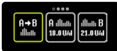
**2/4:** If basal rate profile A is active, tap the “Switch to basal rate profile B” icon.
