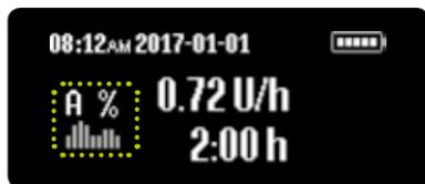
**6/7:** The status screen appears with the actual basal rate. A % sign next to the basal rate profile set indicates that a temporary basal rate function is active.
