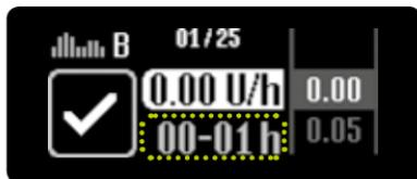
**3/8:** The screen to set the basal rate for the first hour appears, starting at midnight (00–01 h). When putting into operation for the first time (when programming a basal rate profile for the first time), an hourly value, which is set and confirmed, is applied to the next hour as a starting value.
