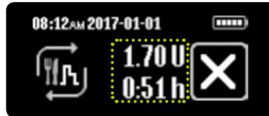
**8/8:** The YpsoPump® counts down the remaining units on the status screen. The immediate portion of the bolus is delivered first. It is followed by the extended portion. In addition, the remaining extension time of the extended bolus is displayed. You can cancel a bolus in progress at any time by tapping . Cancellation must always be confirmed by tapping .
