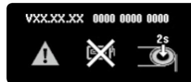
Then press the function button for 2 seconds. The insulin pump is now devoid of a battery and in storage status. To put the insulin pump back into operation perform the steps on page 31 and check your therapy settings. Change the cartridge and the infusion set in accordance with the steps on page 94.
