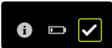
If the “Battery charge level low” warning appears, the YpsoPump® can still be operated for at least two days. Confirm by tapping  and insert a new AAA alkaline battery (LR03) as soon as possible. Follow the procedure on page 140. Having confirmed the warning you will still see the low battery charge on your status screen. The “Battery charge level low” warning escalates to the “Battery empty” alarm if the battery is not changed in the meantime.
