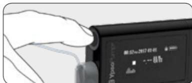
**1/6:** The status screen of the YpsoPump® is switched on and off by pressing the function button (short button press).
