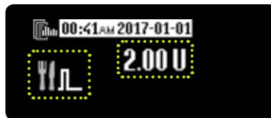
**2/4:** The icon of the bolus type appears on the left of the screen, the relevant value in the middle. The delivery time and delivery date are shown at the top on a white background. By swiping to the left you can quit the display of last bolus at any time and return to the status screen.
