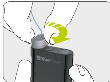
**2/2:** Place the adapter on the inserted cartridge upright. Turn the adapter clockwise to the lock position. You should hear a soft click and/or feel a definite mechanical stop.
