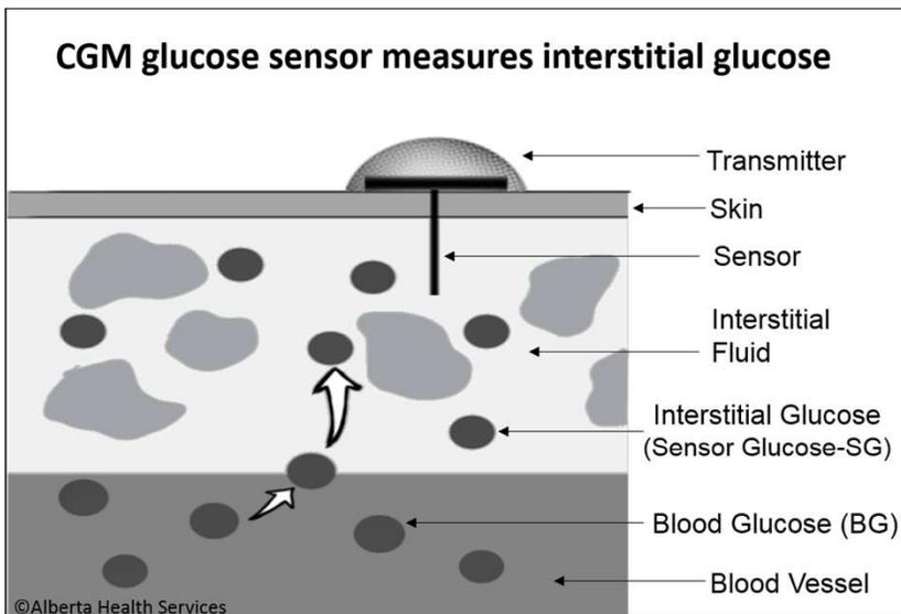
A glucose sensor (small electrode) is inserted under the skin and measures interstitial glucose every 1-5 minutes. The readings are sent wirelessly to a device, either automatically or by manually scanning the sensor with a reader. There are two major types of CGM.
