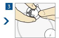
Slide the set release connector into the set connector.
