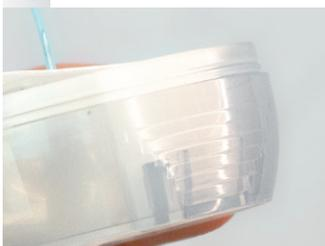
To spring-load the insertion device, place your fingers on the lined ridges on both sides of the device and press in.
